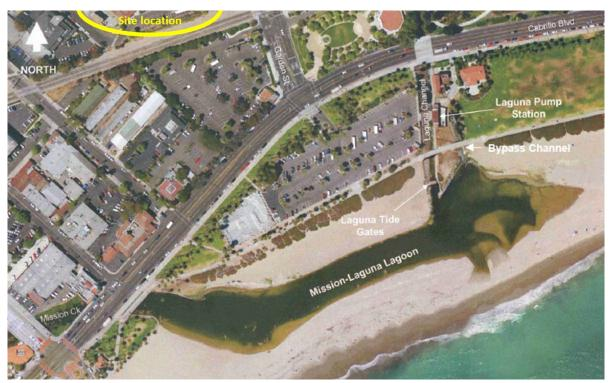
Figure 4. Depiction of the Laguna Channel Pump Station, Bypass Channel, Tide Gates, and Lagoon. Adapted from CA Coastal Commission (https://documents.coastal.ca.gov/reports/2006/6/T23b-6-2006.pdf),
