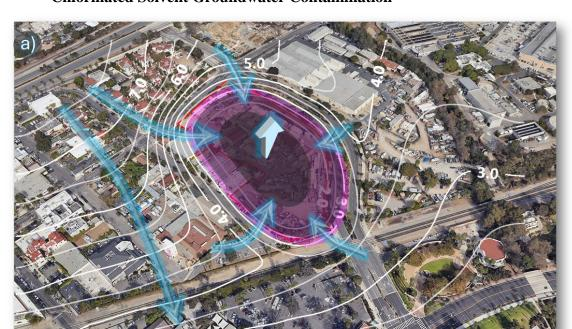
Figure 3: Impacts of Construction Dewatering to the Subsurface Redistribution of Chlorinated Solvent Groundwater Contamination
